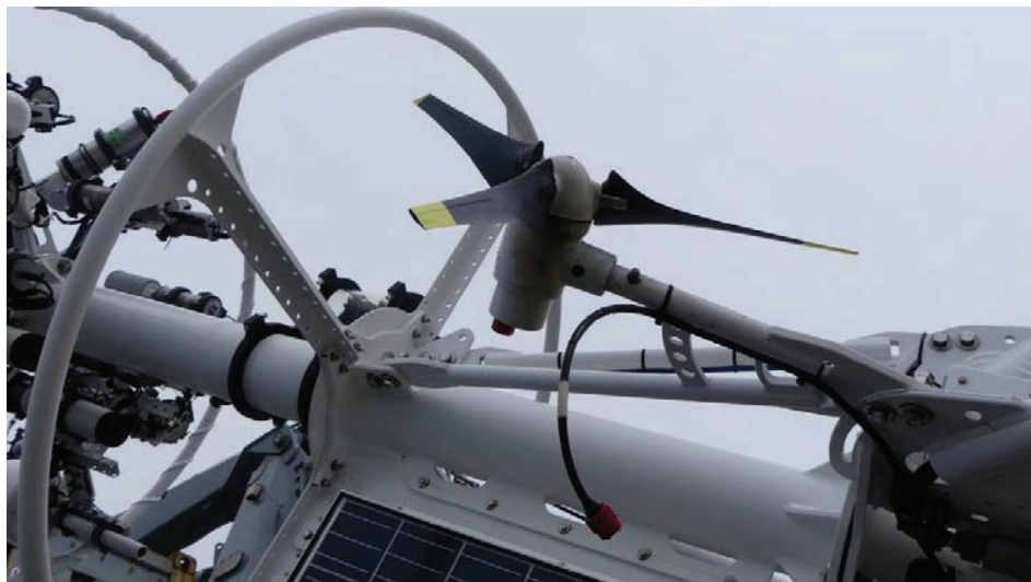
Figure 3-36 – The starboard wind turbine was unplugged and all 3 blade tips were broken off
