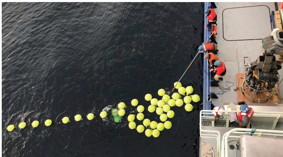
Figure 3-31 – Hooking into the glass balls from the GI01SUMO-00005 mooring
