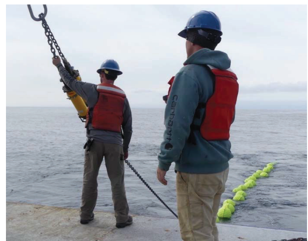
Figure 3-28 – Deployment of GI03FLMB-00006 OSNAP instruments and acoustic releases
