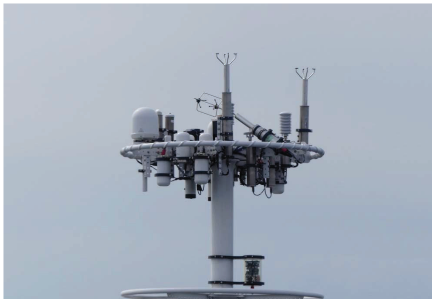
Figure 3-34 – The FDCHP was leaning back on the starboard METBK BPR
