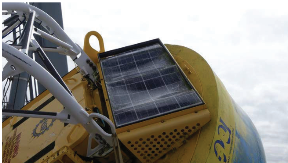
Figure 3-37 – The starboard PV panel was smashed and warped
