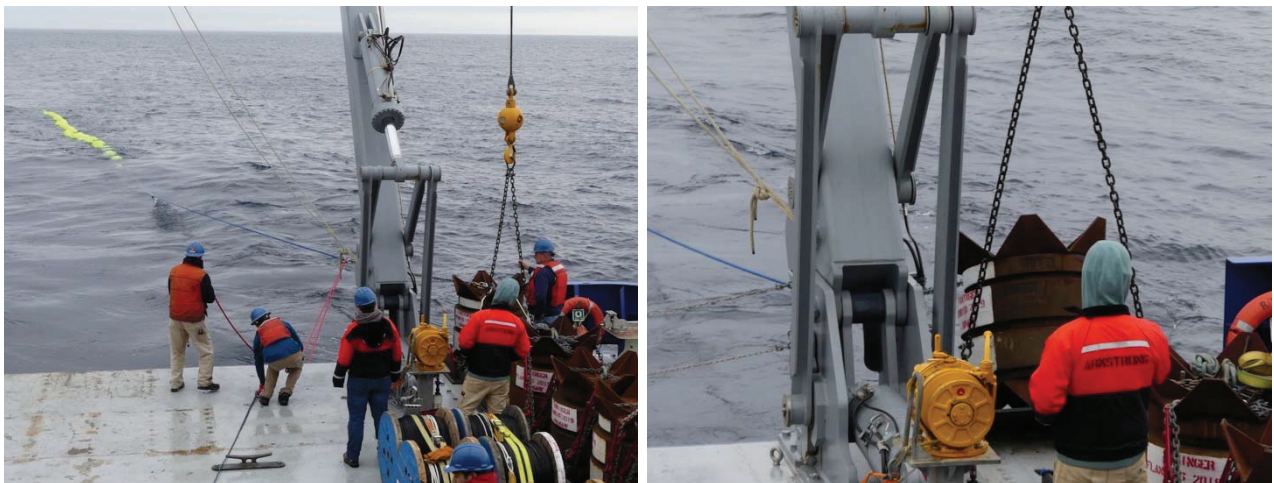
Figure 3-16 – Shifting the load to, and deploying the GI02HYPM-00006 anchor
