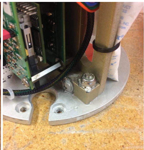
Figure 3-51 – GI03FLMB-00005 Main controller corrosion
