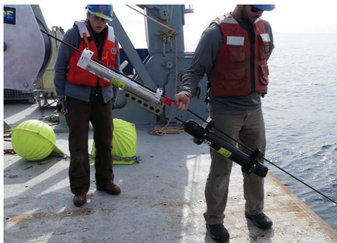
Figure 3-28 – Deployment of GI03FLMB-00006 OSNAP instruments and acoustic releases
