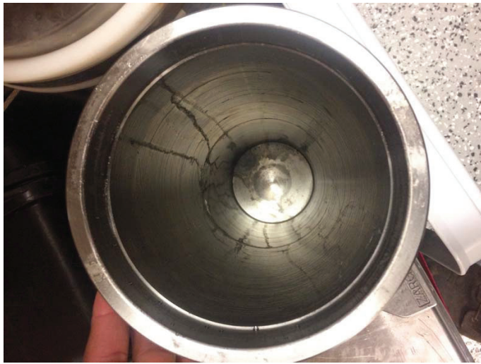
Figure 3-50 – GI03FLMB-00005 Main controller housing leak and corrosion
