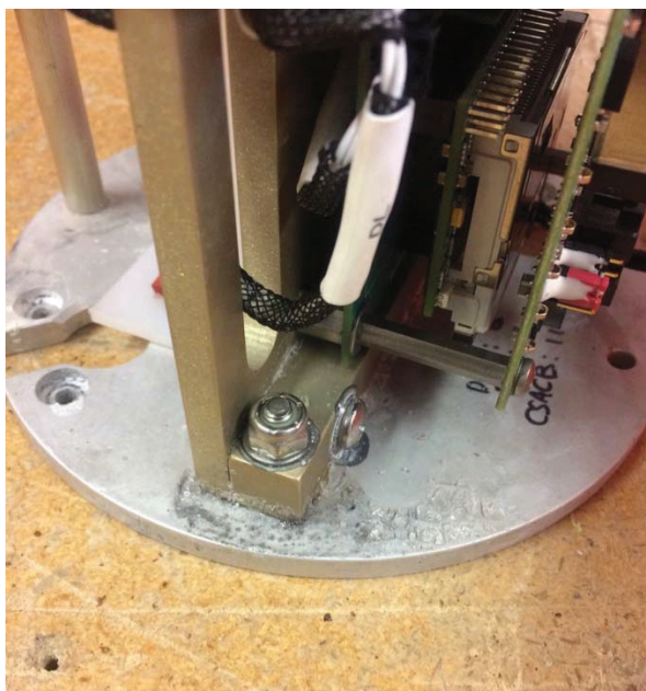
Figure 3-51 – GI03FLMB-00005 Main controller corrosion
