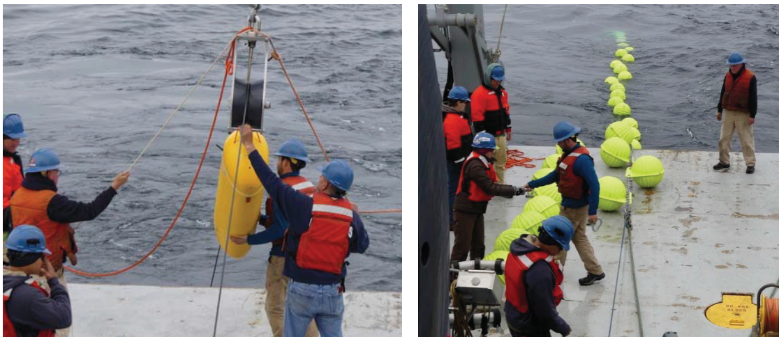
Figure 3-15 – Deployment of the GI02HYPM-00006 WFP (left) and glass balls (right)
