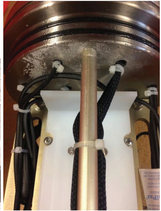
Figure 3-50 – GI03FLMB-00005 Main controller housing leak and corrosion
